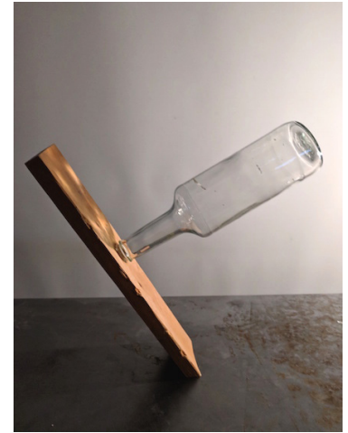
Figure 8.8: If the center-of-mass of an object is above the base of its support, it will balance. This bottle and board, constructed by Prof. Rhett Zollinger, demonstrates this dramatically. The combined center of mass for this glass bottle and wood board is position directly over the board's small edge, allowing it to balance.
